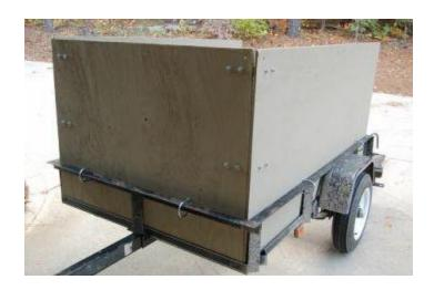
Step 4: Attach tarp. Note that in this picture, attachment points have been screwed into the plywood on the sides (and in the front) to attach bungee cords to tension the tarp. Apply other bungees as needed to wind-proof the tarp. Loading can be done after the tarp is on in case of bad weather. Then close ramp, drape tarp over it and bungee.
