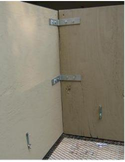
Step 3: The u-bolts were attached around the frame, and through the plywood where they were affixed with wing nuts. The u-bolts were cut down a bit so that the ends of the bolts wouldn't damage any of the material being moved in the trailer
