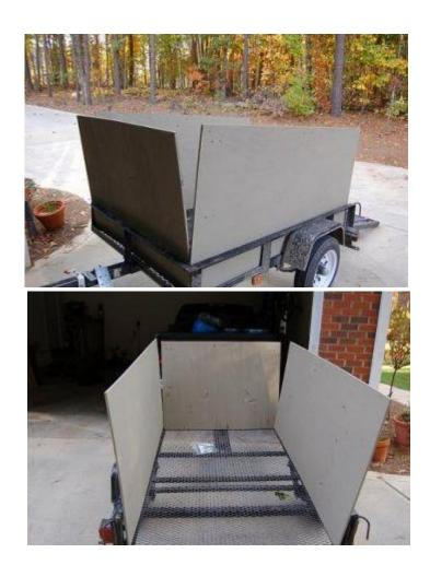
Step 2: I used drilled holes to make sure I lined up the front piece with the appropriate side piece so the angle brackets would match the pre-drilled holes. Then the angle brackets are bolted into position finger tight.
